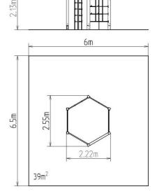
The support structure of the climbing set is made of structural steel which is protected against corrosion by zinc coating, resulting in a very prolonged service life of the workout elements or duplex powder coated with coat curing according to RAL to prevent corrosion. All other metallic elements are also zinc coated or duplex powder coated with coat curing according to RAL to prevent corrosion.
