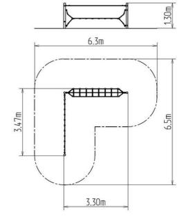
The support structures of the rope unit are made from structural steel, they are zinc coated or duplex powder coated with coat curing according to RAL to prevent corrosion and fixed in a concrete bed. The support structures can be hot-dip galvanized should the client require. The ropes are made using HERKULES material (16 mm thick ropes made from polypropylene with a steel internal core) and are connected with plastic joints. All fastening material is galvanized or stainless steel.
