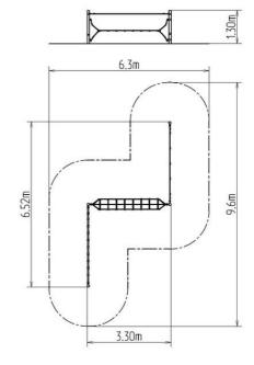
The support structures of the rope unit are made from structural steel, they are zinc coated or duplex powder coated with coat curing according to RAL to prevent corrosion and fixed in a concrete bed. The ropes are made using HERKULES material (16 mm thick ropes made from polypropylene with a steel internal core) and are connected with plastic joints. All fastening material is galvanized or stainless steel.
