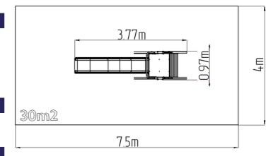
The support structure of the slide is made from structural steel, which is zinc coated or duplex powder coated with coat curing according to RAL to prevent corrosion and is fixed in a concrete bed. All metal units are zinc coated or duplex powder coated with coat curing according to RAL to prevent corrosion.
