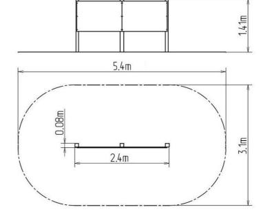
The support structure of the drawing board is made of structural steel which is protected against corrosion by zinc coating, resulting in a very prolonged service life of the workout elements or duplex powder coated with coat curing according to RAL to prevent corrosion. These structures are anchored to concrete footings. All other metallic elements are also zinc coated or duplex powder coated with coat curing according to RAL to prevent corrosion.
