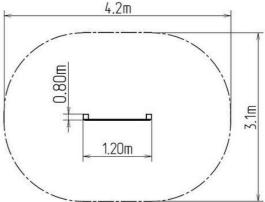
The supporting structure of the tear bar is made of structural steel (60 x 60 mm metal profile), which is protected against corrosion by a zinc coating, which results in a very significant prolongation of the play element lifetime and fired by KOMAXIT RAL. These structures are embedded in a concrete bed. All other metal elements are also treated with galvanizing and fired with KOMAXIT RAL.
