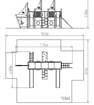
The support structure of the tower unit is made of structural steel which is protected against corrosion by zinc coating, resulting in a very prolonged service life or duplex powder coated with coat curing according to RAL to prevent corrosion. All other metallic elements are also zinc coated or duplex powder coated with coat curing according to RAL to prevent corrosion.
