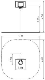
The basketball basket support structures is made from structural steel, protected from corrosion by hot-dip galvanizing, which significantly prolongs the life of the play unit. The structures are fixed in a concrete bed. The basketball board is made from water-proof plywood designed for external use. All fastening material is galvanized or stainless steel.
