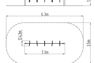
The support structures of the rope unit are made from structural steel, they are zinc coated or duplex powder coated with coat curing according to RAL to prevent corrosion and fixed in a concrete bed. The ropes are made using HERKULES material (16 mm thick ropes made from polypropylene with a steel internal core) and are connected with plastic joints. All fastening material is galvanized or stainless steel.
