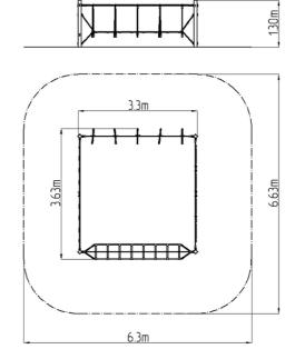
The support structures of the rope unit are made from structural steel, they are zinc coated or duplex powder coated with coat curing according to RAL to prevent corrosion and fixed in a concrete bed. The ropes are made using HERKULES material (16 mm thick ropes made from polypropylene with a steel internal core) and are connected with plastic joints. All fastening material is galvanized or stainless steel.
