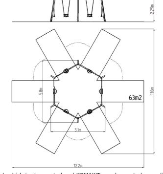
The support structure of the swing is made from structural steel, which is zinc coated and KOMAXIT powder coated according to the RAL colour chart. The structures are anchored into the ground in steel plates, which are protected against corrosion by hot-dip galvanizing a and fixed in a concrete bed. The anchors are fastened to the play unit with bolts and their structure ensures that they are not in direct contact with the ground.
