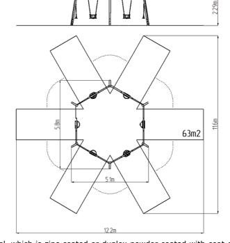
The support structure of the swing is made from structural steel, which is zinc coated or duplex powder coated with coat curing according to RAL to prevent corrosion. The structures are anchored into the ground in steel plates, which are protected against corrosion by hot-dip galvanizing a and fixed in a concrete bed. The anchors are fastened to the play unit with bolts and their structure ensures that they are not in direct contact with the ground.
