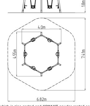
The support structure of the swing is made from structural steel, which is zinc coated and KOMAXIT powder coated according to the RAL colour chart. The structures are anchored into the ground in steel plates, which are protected against corrosion by hot-dip galvanizing a and fixed in a concrete bed. The anchors are fastened to the play unit with bolts and their structure ensures that they are not in direct contact with the ground.
