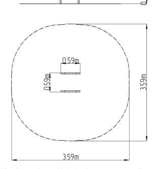
All metal elements such as handles, parallel bars, etc. are treated by zinc coating and baked paint KOMAXIT according to the RAL shade, or according to the customer's request the elements can be made in stainless steel. These structures are anchored to concrete feet. All fasteners are galvanized or stainless steel.
