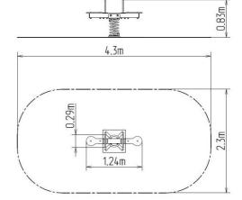
Metal units - structural steel Seats - HPL Spring - special spring steel
