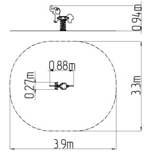
The body of the rocker and the seat are made from high quality HDPE plastic (high density coloured polyethylene, which is characterised by high colour stability, UV resistance but mainly safety as it doesn't break and therefore there is no danger of injury to children by sharp fragments). The swing spring is made from special spring steel and duplex powder coated with coat curing according to RAL to prevent corrosion. All fastening material is galvanized or stainless steel.
