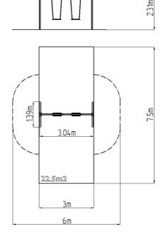
The support structure of the swing is made from structural steel, which is zinc coated or duplex powder coated with coat curing according to RAL to prevent corrosion and is fixed in a concrete bed. The Normal seat is made of aluminum, covered with a soft and comfortable rubber. The chains are stainless steel, resulting in a very prolonged service life of the product. All fastening material is galvanized or stainless steel.
