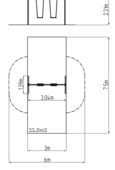
The support structure of the swing is made from structural steel, which is zinc coated or duplex powder coated with coat curing according to RAL to prevent corrosion and is fixed in a concrete bed. The Normal seat is made of aluminum, covered with a soft and comfortable rubber. The chains are stainless steel, resulting in a very prolonged service life of the product. All fastening material is galvanized or stainless steel.
